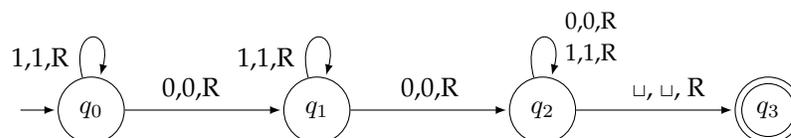
The language in question is regular, so we can build a DFA for it. We can convert it to a Turing Machine by basically leaving the tape alone and always moving right. This sort of thing works to turn any DFA into a Turing Machine.
