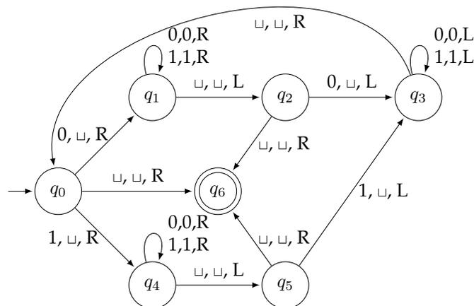
Consider a palindrome like 0010100. Notice how the first and last symbols must match, as must the second and second-to-last, etc. This suggests that our Turing Machine look at the first character, erase it, scan to the right until the end of the string, and compare the last to the first. Then it can move back to the left and repeat the process.
