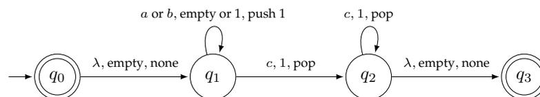
The notation on the loop on  $q_1$  is a shorthand for four possible transitions: if the current input symbol is an  $a$  or a  $b$  and there is a 1 on top of the stack or the stack is empty, then stay at  $q_1$  and push a 1 onto the stack. For parts (a), (b), and (c), assume that the transition from  $q_0$  to  $q_1$  is always taken.
