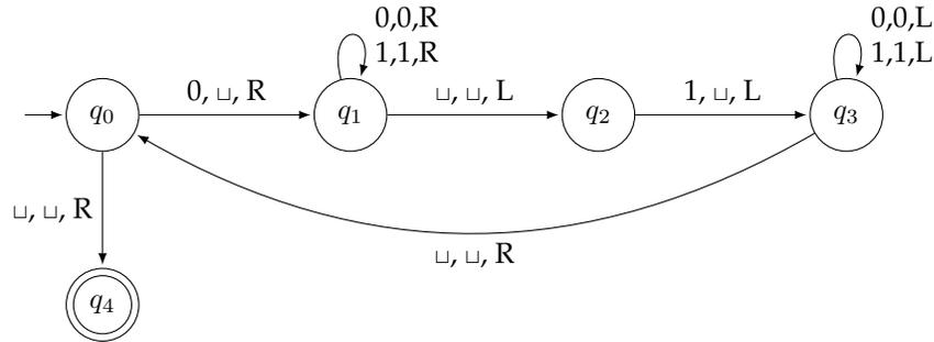
A diagram like this can be a little overwhelming to understand at first glance. Behind the diagram there lies a simple strategy. We start by erasing the first 0. Then we scan right until we get to the last 1 and erase it. Then we scan back left and erase the first 0, and we keep scanning back and forth, erasing symbols until there's nothing left. If we get to that point, then we accept the string. Here are the first several moves of the machine on the input string 000111:
