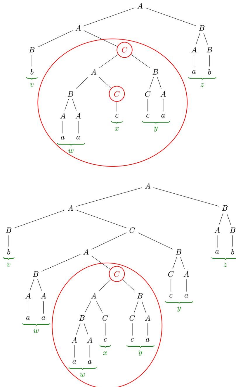
In the first parse tree above, we have broken the input string  $baacacab$  into five parts:  $vwxyz$ . Notice how those parts also show up in the second parse tree, except that  $w$  and  $y$  are repeated. The pasting process
