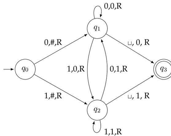
The strategy here is to overwrite the current tape symbol with # initially and with the most recently read tape symbol after that, using the states of the machine to “remember” what that symbol is.
