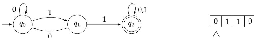
We feed this machine an input string like 0110. We can think of the DFA as consisting of two parts: the state machine (shown above on the left), that acts as the main processor, and an input unit (shown above on the right) with a read head that scans left to right across a tape one symbol at a time, feeding those symbols into the state machine.
