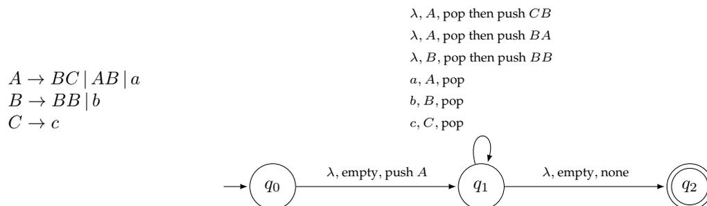
In general, the construction always has exactly 3 states. It always starts with a  $\lambda$  transition that pushes the start variable onto the stack, and it always ends with a transition from the second state to the final state on an empty stack.
