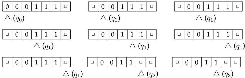
At this point it starts scanning left again at state  $q_3$  until it reaches the left end of the tape (indicated by a blank). It uses the blanks at either end to know when to turn around. We continue scanning back and forth until there is nothing left on the tape but blanks. We recognize this situation at state  $q_0$  if we see only a blank as we try to move right.
