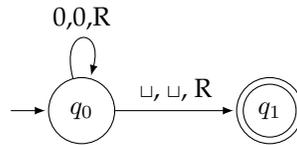
Here is the basic idea behind this machine: Each time we read a 0, we write a 0 (i.e., the tape contents don't change since there already is a 0 there), and move the read head right. If we ever see a nonzero value, there is no transition for that, and the machine automatically rejects the string. If we reach the end of the input, we will see a blank symbol ( $\square$ ). When we see that, we know we're good and we move to the accepting state.
