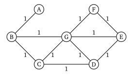
In routing, we are interested in finding the shortest (cheapest) path from one router/vertex to another. For instance, there are many paths from *A* to *E* in the graph above. We could route packets along the long path  $A \rightarrow B \rightarrow C \rightarrow G \rightarrow F \rightarrow E$ , but it's cheaper to go  $A \rightarrow B \rightarrow G \rightarrow E$  for a cost of 3.
