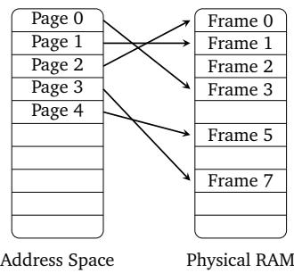
Notice in particular, that the frame for a page can be anywhere. Things don't have to go in any particular order. Frame 4 in the figure above doesn't have a page corresponding to it, but it might correspond to some other process's page. In general, each process has its own set of mappings.
