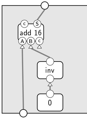
The idea is simply that we need to add the value  $a$  with 1. To get 1, we can use the 0 component (that is always 0) followed by an invert component to make it 1.
