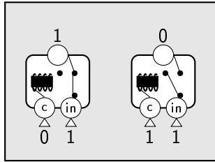
Since NAND is NOT AND, we can connect the first relay to the second one like below to build a NAND gate.
