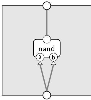
Now that we've built an inverter, just like with the NAND gate, we can put our inverter circuitry into a little box called "inv", and whenever we want to flip a bit, we can plug it into our inverter.
