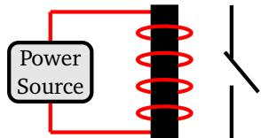
The purpose of a relay is that it acts a little like a light switch, except that instead of being controlled by a person flipping the switch, it is controlled by electric current, basically whether or not the coiled wire is connected to the battery or not.
