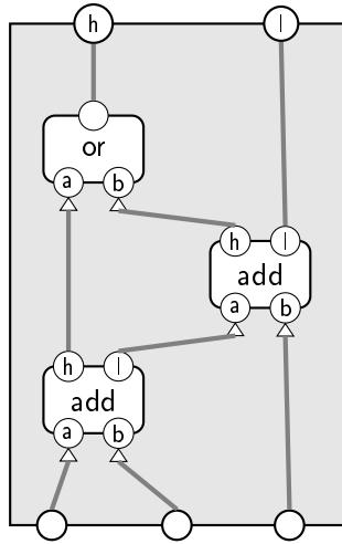
The half-adder on the left adds  $a$  and  $b$ . The low bit of the result gets added with  $c$  in the right adder. The low bit of that is the low bit of the addition  $a + b + c$ . For the high bit, we might get a carry out from either adder. If one or the other or both has a carry, then there will be a carry in the final result, so we use an OR gate to handle that.
