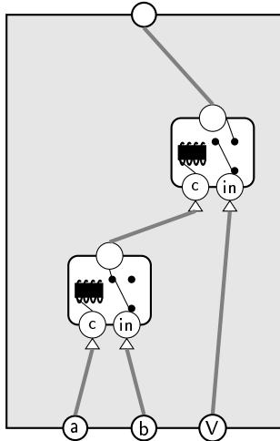
Once we've built the NAND gate, we can imagine packaging it into a little black box labelled NAND and not worry about the relays inside. We can then wire various NAND gates together to do interesting things.
