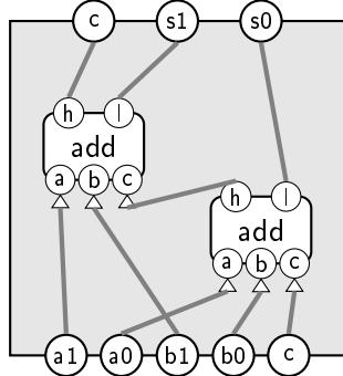
The idea is that we add the right bits and carry first with an adder. This gives us the low bit of the answer. It also might give us a carry. We then add that carry along with the high bits in another adder. Basically, we just add bit-by-bit, taking into account the carries.
